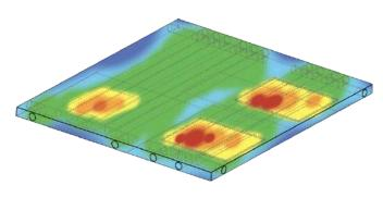
**CLCP** includes multi-channel cold water inlet/outlet owning high flexibility in adjusting numbers of inlet/outlet (up to 4in 4out) by request. When coolant flows through top sink, liquid can absorb the heat and take it away from the heat sources quickly to the heat exchanger. When heated liquid flushes into the heat exchanger, it will be cooled by 9 units of 12 x 12 cm active fan which can run at 2K~3K RPM.
